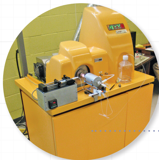
Scott Tanner and his team developed mass cytometry, also known as CyTOF, employing metal-tagged antibodies to label and identify proteins on individual cells. In 2009, the first commercial CyTOF instrument by DVS Sciences started operating in Tanner's laboratory.
